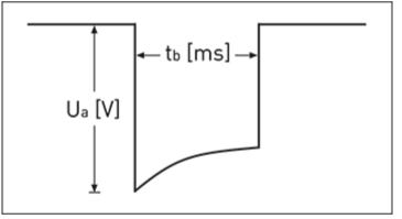
The pulse amplitude reaches its maximum value at the beginning of the pulse (Ua). With increasing pacing duration (tb), the pulse amplitude is reduced dependent on the pacing impedance.
