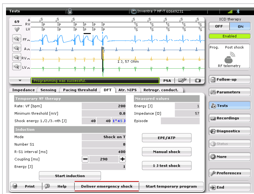
Figure 197: DFT screen with 1 J Test Shock being delivered
