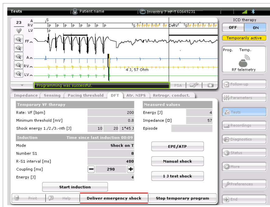
Figure 201: Shock-on-T Induction (the shock waveform for induction is biphasic)
